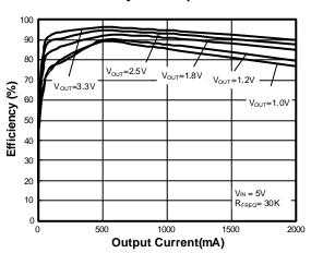
**Efficiency vs. Output Current**
