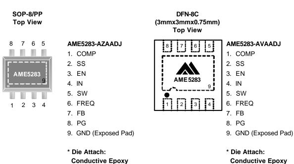
Note. Connect exposed pad (heat sink on the back) to GND.
