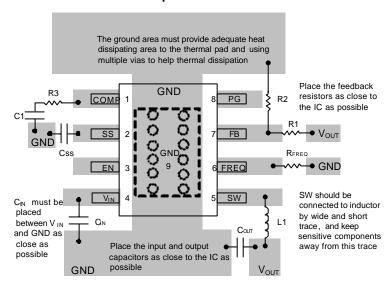
Figure 3. AME5283 Regulators Layout Diagram
