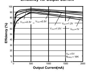
**Efficiency vs. Output Current**
