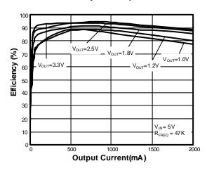
**Efficiency vs. Output Current**
